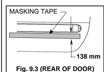
At the leading edge of the door, locate a small piece of masking tape so that its upper edge is 137 mm up from the lower door edge. At the back of the door, locate another small piece of masking tape 138 mm up from the lower door edge.
