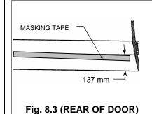
At the leading edge of the door, locate a small piece of masking tape so that its upper edge is 135 mm up from the lower door edge. At the back of the door, locate another small piece of masking tape 137 mm up from the lower door edge. At the Midpoint of the door locate a third small piece of masking tape 136 mm up from the lower door edge.
